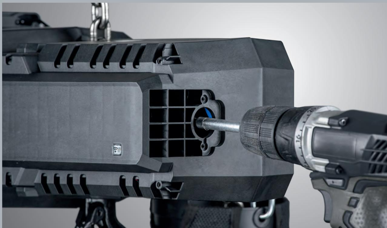
If the battery runs out during hoist operation, the load can be manually lowered. Simply open the end compartment and use a screwdriver or power drill to lower the load.
