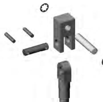
Figure 11. 3 Ton (3000 kg) Hoist to Trolley Assembly
