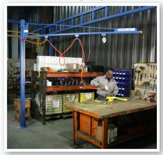
The TSJ50 is designed for easy movement of light loads. Its lightweight tie rod style insures easy movement and high performance without giving you more crane than you need for low capacity applications.
