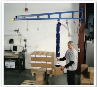
For heavier or higher impact applications, Gorbel offers the TSJ150. The lightweight design makes this higher capacity tool jib easy to operate as either a free standing or a column/wall mounted style.
