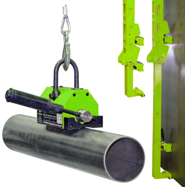
**Picture above right:** A customized version of IMI's Vertical Lift Adaptor featuring two PowerLift® magnets, designed to lift ferrous metal from horizontal to vertical orientation or vice versa. Adjustable for various widths, thicknesses and shapes. Ask for a PowerLift Tech Sheet for specifications.
