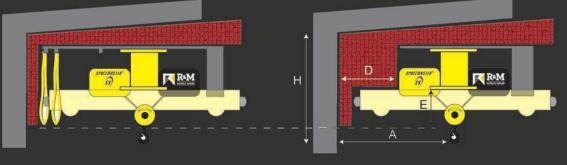
Potential space savings when using R&M's QX modular crane package versus competitors cranes (Figure 1) and the added space savings versus standard C-track festoon system cranes (Figure 2)
