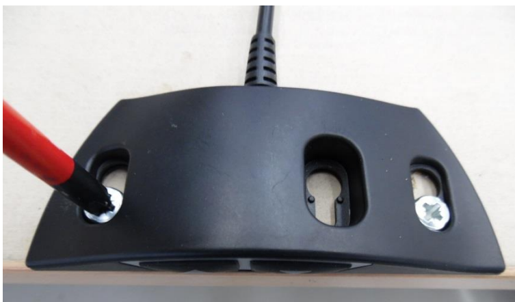
Figure 13 Attaching the simple manual switch UBM-F/2-p
