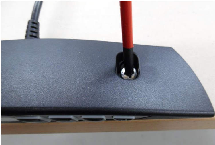
Figure 15 Attaching of the programmable manual switch UBS/6-LCD
