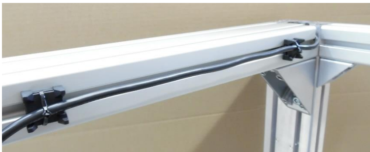
Figure 23 Cable guide with cable holders
