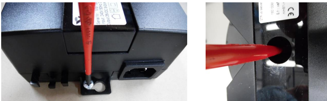
Figure 15 Attaching the electrical controller (screw linkages: left 3x, right 1x)
