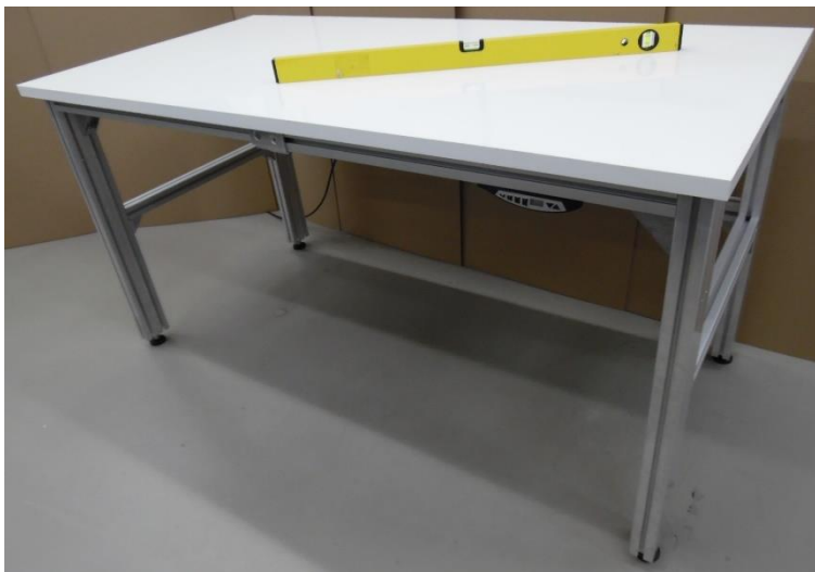
Figure 25 Adjusting the workplace with a spirit level
