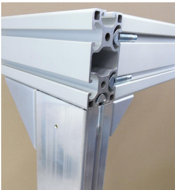
Figure 9 Supporting connection of base frame on the frontal outer profile of the lifting elements
