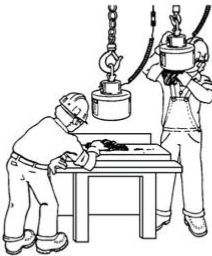
Check the condition of the magnet prior to every lift.
