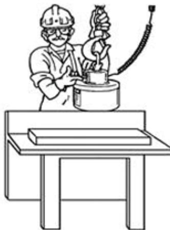
Carefully set the load down. De-energize the magnet by selecting the **"PROOF"** & **"RELEASE."** The red indicator light will flash. Hold for two to three seconds; when released the magnet will return to the **"OFF"** position. Then lift the magnet slightly to be sure the load has been released.
