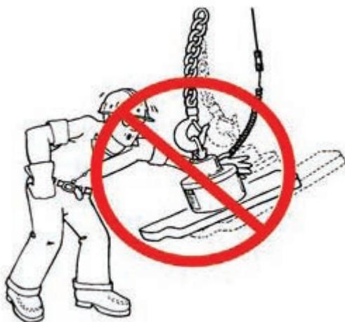
Lift and move the load SMOOTHLY. Avoid jarring and swinging the load while it is in transit. KEEP THE LOAD LEVEL. NEVER let the load come in contact with any obstruction.
