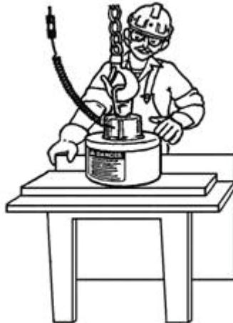
Energize the magnet by selecting the **"GRIP" & "PROOF buttons**. The green indicator light will illuminate when electrical power is applied to the magnet. To obtain maximum lift, allow a few seconds for the magnet to reach full power before lifting the load.
