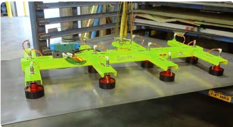
The Magnetic Sheet Lifter features a series of permanent magnetic lifting heads to lift a wide variety of sheet lengths and widths. On-board or remote controls are provided to control pneumatic cylinders that are located on the magnetic heads. Once activated, the cylinders move the magnets in a housing and grip or release the sheet from or to its desired location.
