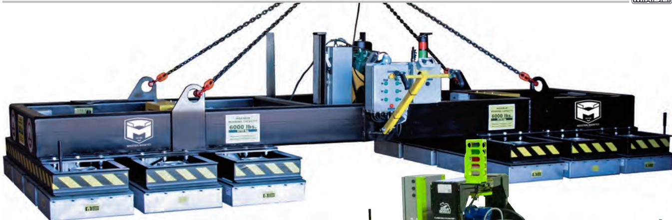
The Magnetic Sheet Lifter de-stacks steel sheets from pallets, racks and more. The unique design of this permanent magnetic lifting system allows one person to safely and effectively move and load sheets onto cutting tables, shear beds and other fabrication equipment.
