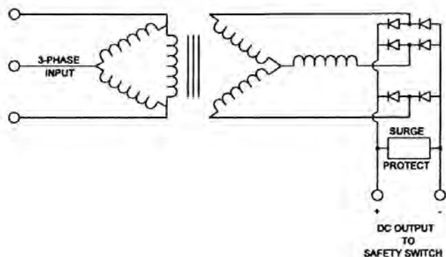
Rectifier must be rated for magnet service and be equipped with surge protection.
